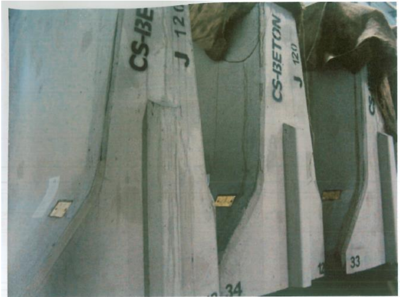
Figure 15 – Marking with paint on every part front
