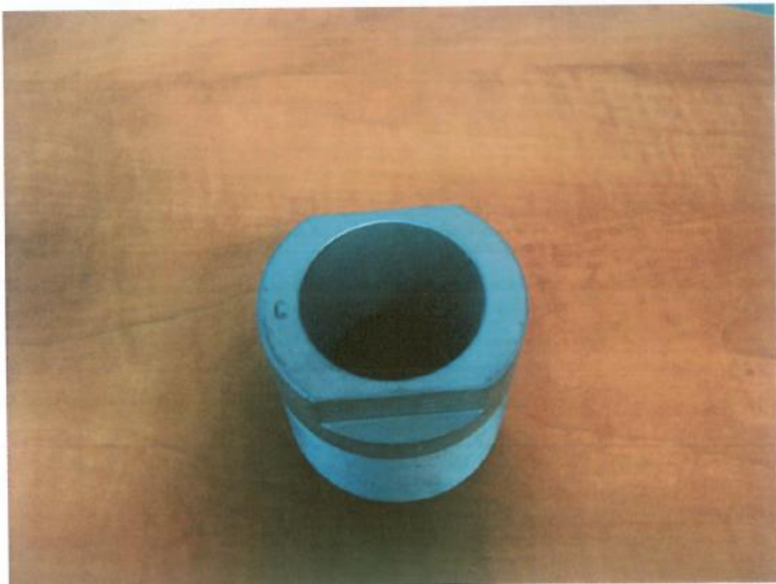
Figure 14 – Marking of coupling
